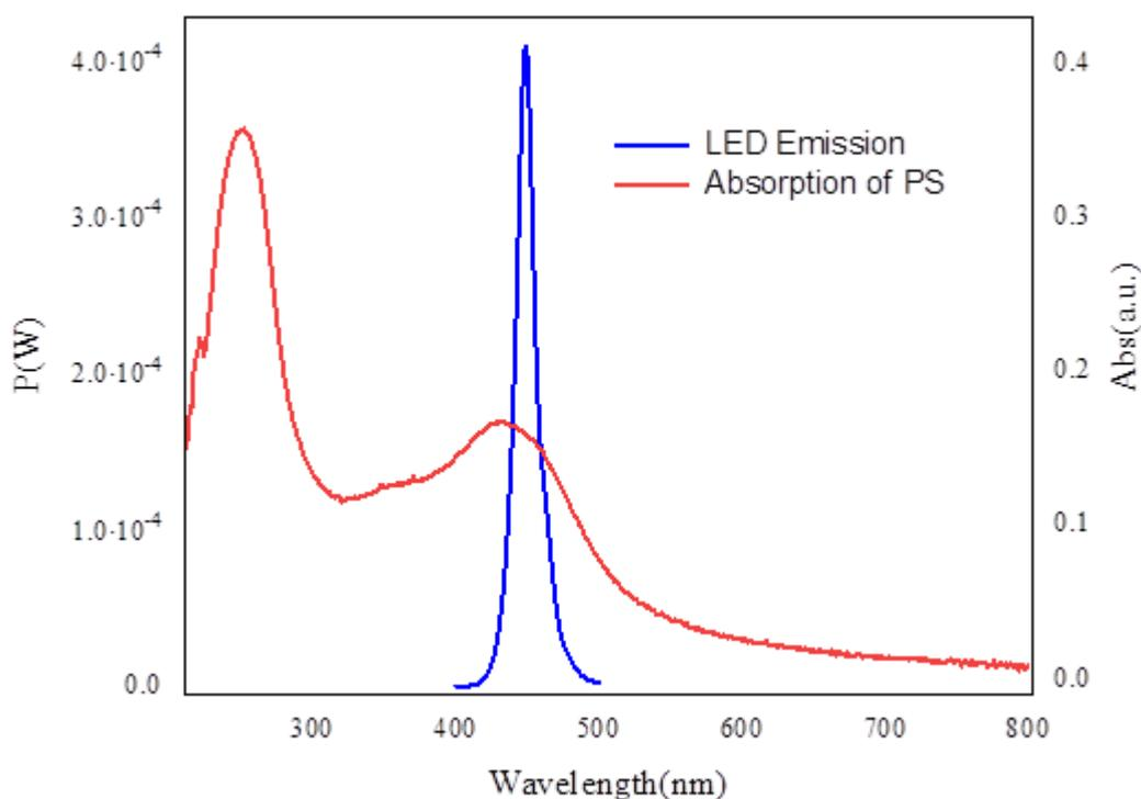
**Figure 1.** Light-emitting diode emitted potency ( $P_{LED}$  emitted) and PS electronic absorption spectra.
